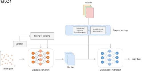
Figure 6: Architecture of a CTGAN model [3].
